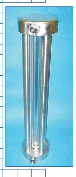
The Chem Flowtronics Series LG-1160 Sanitary Level Gauge offers 360-degree view of the process fluid for liquid level verification, and process validation. Chemflowtronics unique end fittings with integral 90 degree elbows, reduces process dead space, increases tank visual verification area, and eliminates the leak paths associated with secondary fittings.
