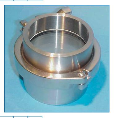
Chem Flowtronics unique Sanitary design sightglasses designed using standard sanitary piping components modified to support BOROSILICATE safety glass lens. The unique design criteria offers a small retention area above the lens to eliminate the retention areas thus increasing cleanability.
